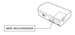
**2** Slide the mode switch to the "AP" side, press the power button to turn the device on.
