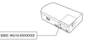
**2** Slide the mode switch to the "AP" side, press the power button to turn the device on.
